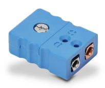
ProSense Type T thermocouple connector, standard round pin jack, 400 deg F (200 deg C), glass filled thermoplastic body, blue, thermocouple material pins, 32 AWG to 14 AWG wire size range.
