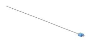
ProSense temperature sensor, Type T thermocouple, attached plug probe, ungrounded, 18in insertion length, 1/8in probe diameter, stainless steel sheath, 2-pin miniature size plug.
