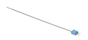
ProSense temperature sensor, Type T thermocouple, attached plug probe, ungrounded, 12in insertion length, 1/8in probe diameter, stainless steel sheath, 2-pin miniature size plug.
