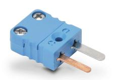
ProSense Type T thermocouple connector, miniature flat pin plug, 400 deg F (200 deg C), glass filled thermoplastic body, blue, thermocouple material pins, 40 AWG to 20 AWG wire size range.
