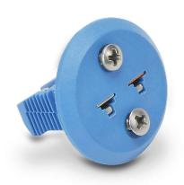
ProSense Type T thermocouple connector, miniature flat pin panel jack, 400 deg F (200 deg C), glass filled thermoplastic body, blue, thermocouple material pins, 32 AWG to 14 AWG wire size range.
