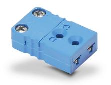
ProSense Type T thermocouple connector, miniature flat pin jack, 400 deg F (200 deg C), glass filled thermoplastic body, blue, thermocouple material pins, 40 AWG to 20 AWG wire size range.
