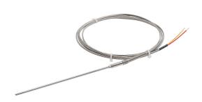
ProSense temperature sensor, Type K thermocouple, lead wire transition probe, ungrounded, 18in insertion length, 1/8in probe diameter, stainless steel sheath, 6ft 20 AWG wire leads.
