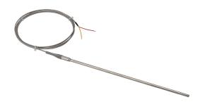
ProSense temperature sensor, Type K thermocouple, lead wire transition probe, ungrounded, 12in insertion length, 1/4in probe diameter, Inconel Alloy 600 sheath, 6ft 20 AWG wire leads.
