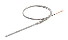
ProSense temperature sensor, Type K thermocouple, lead wire transition probe, ungrounded, 12in insertion length, 1/4in probe diameter, stainless steel sheath, 6ft 20 AWG wire leads.
