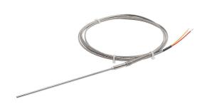
ProSense temperature sensor, Type K thermocouple, lead wire transition probe, ungrounded, 12in insertion length, 1/8in probe diameter, stainless steel sheath, 6ft 20 AWG wire leads.
