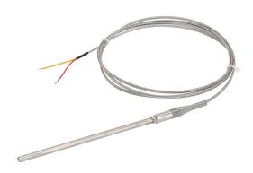
ProSense temperature sensor, Type K thermocouple, lead wire transition probe, ungrounded, 6in insertion length, 1/4in probe diameter, Inconel Alloy 600 sheath, 6ft 20 AWG wire leads.
