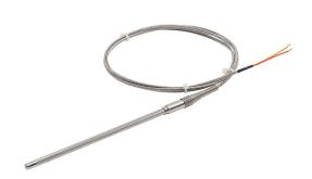
ProSense temperature sensor, Type K thermocouple, lead wire transition probe, ungrounded, 6in insertion length, 1/4in probe diameter, stainless steel sheath, 6ft 20 AWG wire leads.
