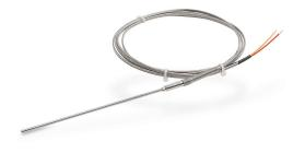
ProSense temperature sensor, Type K thermocouple, lead wire transition probe, ungrounded, 6in insertion length, 1/8in probe diameter, stainless steel sheath, 6ft 20 AWG wire leads.
