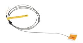
ProSense temperature sensor, Type K thermocouple, spade sensor, ungrounded junction, flexible polyimide with adhesive tape backing, 6ft 24 AWG wire leads.
