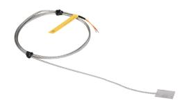
ProSense temperature sensor, Type K thermocouple, spade sensor, grounded junction, stainless steel, 6ft 20 AWG wire leads.
