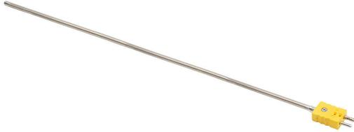
ProSense temperature sensor, Type K thermocouple, attached plug probe, ungrounded, 18in insertion length, 1/4in probe diameter, stainless steel sheath, 2-pin standard size plug.
