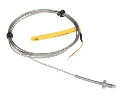
ProSense temperature sensor, Type K thermocouple, threaded bolt sensor, ungrounded junction, 3/8in bolt length, 3/16in tip, stainless steel sheath, 1/4-28 UNF process connection, 6ft 24 AWG wire leads.
