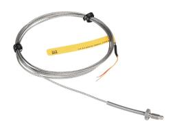
ProSense temperature sensor, Type K thermocouple, threaded bolt sensor, ungrounded junction, 3/8in bolt length, 3/16in tip, stainless steel sheath, 1/4-28 UNF process connection, 6ft 24 AWG wire leads.
