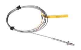
ProSense temperature sensor, Type K thermocouple, threaded bolt sensor, grounded junction, 3/8in bolt length, 3/16in tip, stainless steel sheath, 1/4-28 UNF process connection, 6ft 24 AWG wire leads.
