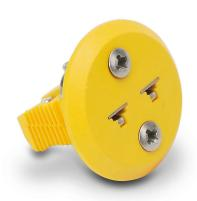
ProSense Type K thermocouple connector, miniature flat pin panel jack, 400 deg F (200 deg C), glass filled thermoplastic body, yellow, thermocouple material pins, 32 AWG to 14 AWG wire size range.
