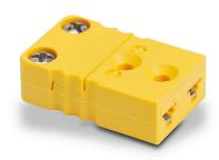
ProSense Type K thermocouple connector, miniature flat pin jack, 400 deg F (200 deg C), glass filled thermoplastic body, yellow, thermocouple material pins, 40 AWG to 20 AWG wire size range.
