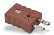
ProSense Type K thermocouple connector, high-temperature standard round pin plug, 662 deg F (350 deg C), glass filled thermoplastic body, brown, thermocouple material pins, 32 AWG to 14 AWG wire size range.
