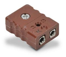
ProSense Type K thermocouple connector, high-temperature standard round pin jack, 662 deg F (350 deg C), glass filled thermoplastic body, brown, thermocouple material pins, 32 AWG to 14 AWG wire size range.
