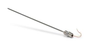
ProSense temperature sensor, Type K thermocouple, hex nipple probe, ungrounded, 18in insertion length, 1/4in probe diameter, Inconel Alloy 600 sheath, 1/2in male NPT process connection, 1/2in male NPT with 3in 24 AWG wire leads.
