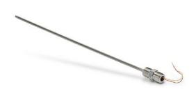
ProSense temperature sensor, Type K thermocouple, hex nipple probe, ungrounded, 18in insertion length, 1/4in probe diameter, Inconel Alloy 600 sheath, 1/2in male NPT process connection, 1/2in male NPT with 3in 24 AWG wire leads.
