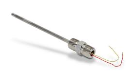
ProSense temperature sensor, Type K thermocouple, hex nipple probe, ungrounded, 6in insertion length, 1/4in probe diameter, Inconel Alloy 600 sheath, 1/2in male NPT process connection, 1/2in male NPT with 3in 24 AWG wire leads.
