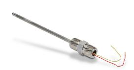
ProSense temperature sensor, Type K thermocouple, hex nipple probe, ungrounded, 6in insertion length, 1/4in probe diameter, Inconel Alloy 600 sheath, 1/2in male NPT process connection, 1/2in male NPT with 3in 24 AWG wire leads.
