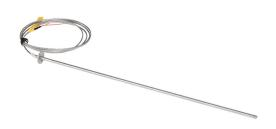
ProSense temperature sensor, Type K thermocouple, flange mount probe, ungrounded junction, 18in insertion length, 1/4in probe diameter, stainless steel sheath, mounting flange process connection, 6ft 20 AWG wire leads.
