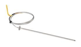
ProSense temperature sensor, Type K thermocouple, flange mount probe, ungrounded junction, 12in insertion length, 1/4in probe diameter, stainless steel sheath, mounting flange process connection, 6ft 20 AWG wire leads.
