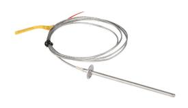
ProSense temperature sensor, Type K thermocouple, flange mount probe, ungrounded junction, 6in insertion length, 1/4in probe diameter, stainless steel sheath, mounting flange process connection, 6ft 20 AWG wire leads.
