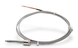
ProSense temperature sensor, Type K thermocouple, spring adjustable immersion probe, grounded, 1/4in insertion length, 3/16in probe diameter, stainless steel sheath, bayonet cap process connection, 10ft 20 AWG wire leads.
