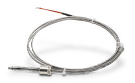
ProSense temperature sensor, Type K thermocouple, spring adjustable immersion probe, grounded, 1/4in insertion length, 3/16in probe diameter, stainless steel sheath, bayonet cap process connection, 6ft 20 AWG wire leads.
