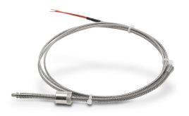
ProSense temperature sensor, Type K thermocouple, spring adjustable immersion probe, grounded, 1/4in insertion length, 3/16in probe diameter, stainless steel sheath, bayonet cap process connection, 4ft 20 AWG wire leads.
