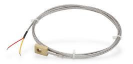
ProSense temperature sensor, Type K thermocouple, bolt-on ring, ungrounded junction, brass sheath, #12, 1/4 - 5/16in (5-8mm) screw or bolt size process connection, 6ft 20 AWG wire leads.
