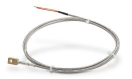
ProSense temperature sensor, Type K thermocouple, bolt-on ring, ungrounded junction, brass sheath, #6 - #10 (4-5mm) screw or bolt size process connection, 6ft 20 AWG wire leads.
