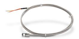
ProSense temperature sensor, Type K thermocouple, bolt-on ring, grounded, stainless steel sheath, #6 to #10 (4mm to 5mm) screw or bolt size process connection, 6ft 20 AWG wire leads.
