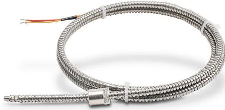
ProSense temperature sensor, Type K thermocouple, armor adjustable immersion probe, grounded, 1/4in insertion length, 3/16in probe diameter, stainless steel sheath, bayonet cap process connection, 4ft 20 AWG wire leads.
