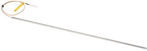
ProSense temperature sensor, Type J thermocouple, cuttable probe, ungrounded junction, 24in insertion length, 1/4in probe diameter, stainless steel sheath, 2ft 20 AWG wire leads.
