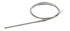
ProSense temperature sensor, Type J thermocouple, lead wire transition probe, ungrounded, 18in insertion length, 1/4in probe diameter, stainless steel sheath, 6ft 20 AWG wire leads.
