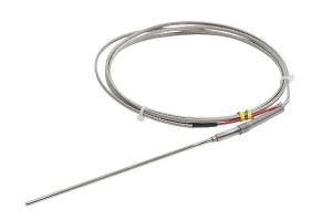
ProSense temperature sensor, Type J thermocouple, lead wire transition probe, ungrounded, 18in insertion length, 1/8in probe diameter, stainless steel sheath, 6ft 20 AWG wire leads.
