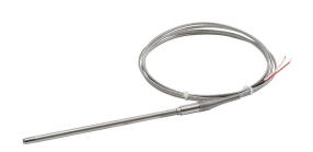
ProSense temperature sensor, Type J thermocouple, lead wire transition probe, ungrounded, 12in insertion length, 1/4in probe diameter, stainless steel sheath, 6ft 20 AWG wire leads.
