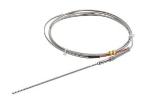
ProSense temperature sensor, Type J thermocouple, lead wire transition probe, ungrounded, 12in insertion length, 1/8in probe diameter, stainless steel sheath, 6ft 20 AWG wire leads.
