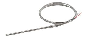
ProSense temperature sensor, Type J thermocouple, lead wire transition probe, ungrounded, 6in insertion length, 1/4in probe diameter, stainless steel sheath, 6ft 20 AWG wire leads.
