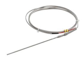
ProSense temperature sensor, Type J thermocouple, lead wire transition probe, ungrounded, 6in insertion length, 1/8in probe diameter, stainless steel sheath, 6ft 20 AWG wire leads.
