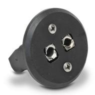
ProSense Type J thermocouple connector, standard round pin panel jack, 400 deg F (200 deg C), glass filled thermoplastic body, black, thermocouple material pins, 32 AWG to 14 AWG wire size range.
