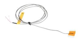
ProSense temperature sensor, Type J thermocouple, spade sensor, ungrounded junction, flexible polyimide with adhesive tape backing, 6ft 24 AWG wire leads.
