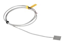
ProSense temperature sensor, Type J thermocouple, spade sensor, grounded junction, stainless steel, 6ft 20 AWG wire leads.
