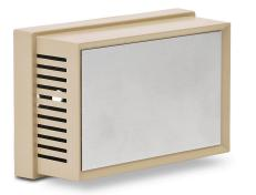
ProSense temperature sensor, Type J thermocouple, room sensor, ungrounded, plastic ventilated housing, metal wall mounting subplate process connection, terminal strip.
