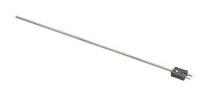
ProSense temperature sensor, Type J thermocouple, attached plug probe, ungrounded, 18in insertion length, 1/4in probe diameter, stainless steel sheath, 2-pin standard size plug.
