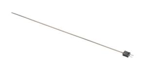
ProSense temperature sensor, Type J thermocouple, attached plug probe, ungrounded, 18in insertion length, 1/8in probe diameter, stainless steel sheath, 2-pin miniature size plug.
