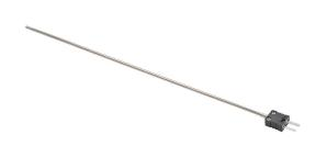
ProSense temperature sensor, Type J thermocouple, attached plug probe, ungrounded, 12in insertion length, 1/8in probe diameter, stainless steel sheath, 2-pin miniature size plug.
