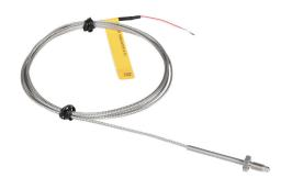
ProSense temperature sensor, Type J thermocouple, threaded bolt sensor, ungrounded junction, 3/8in bolt length, 3/16in tip, stainless steel sheath, 1/4-28 UNF process connection, 6ft 24 AWG wire leads.
