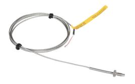
ProSense temperature sensor, Type J thermocouple, threaded bolt sensor, grounded junction, 3/8in bolt length, 3/16in tip, stainless steel sheath, 1/4-28 UNF process connection, 6ft 24 AWG wire leads.
