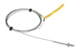
ProSense temperature sensor, Type J thermocouple, threaded bolt sensor, grounded junction, 3/8in bolt length, 3/16in tip, stainless steel sheath, 1/4-28 UNF process connection, 6ft 24 AWG wire leads.
